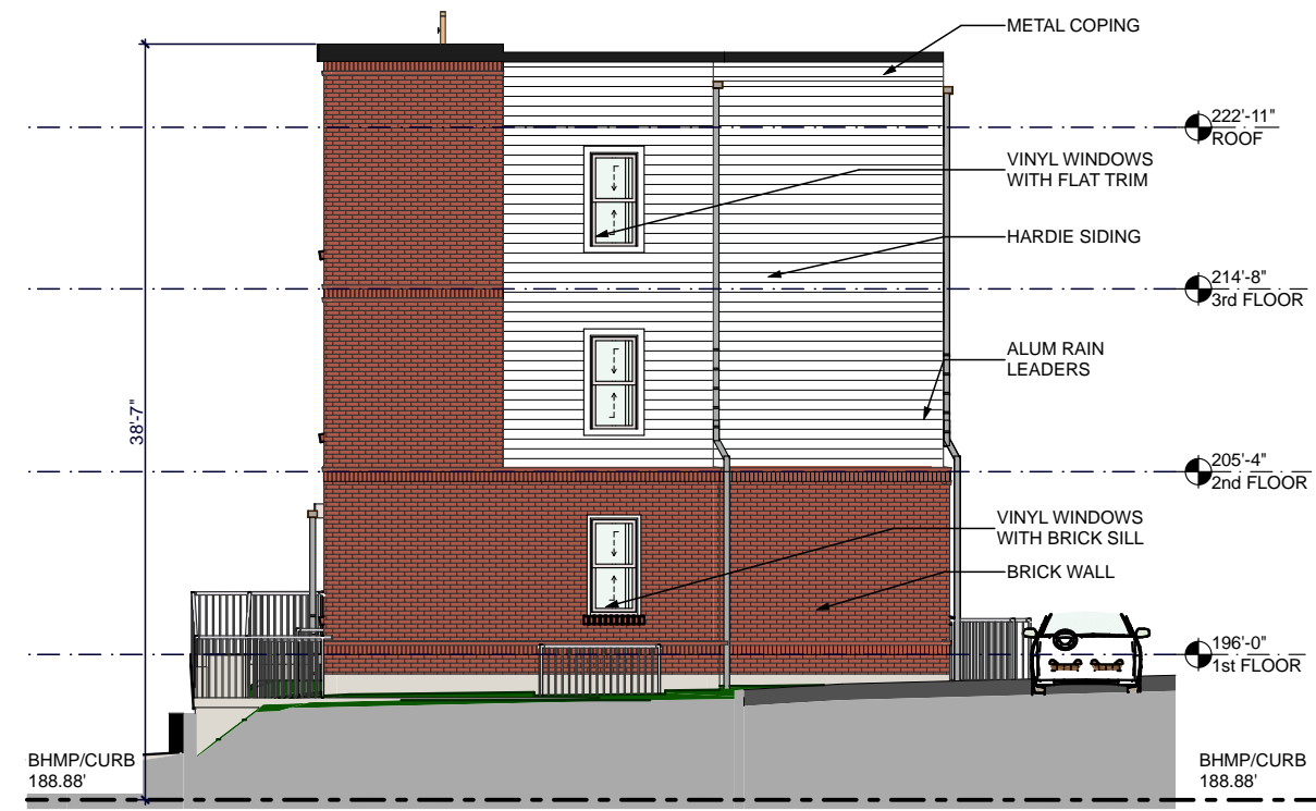
2 NORTH ELEVATION SCALE: 3/32" = 1'-0"
