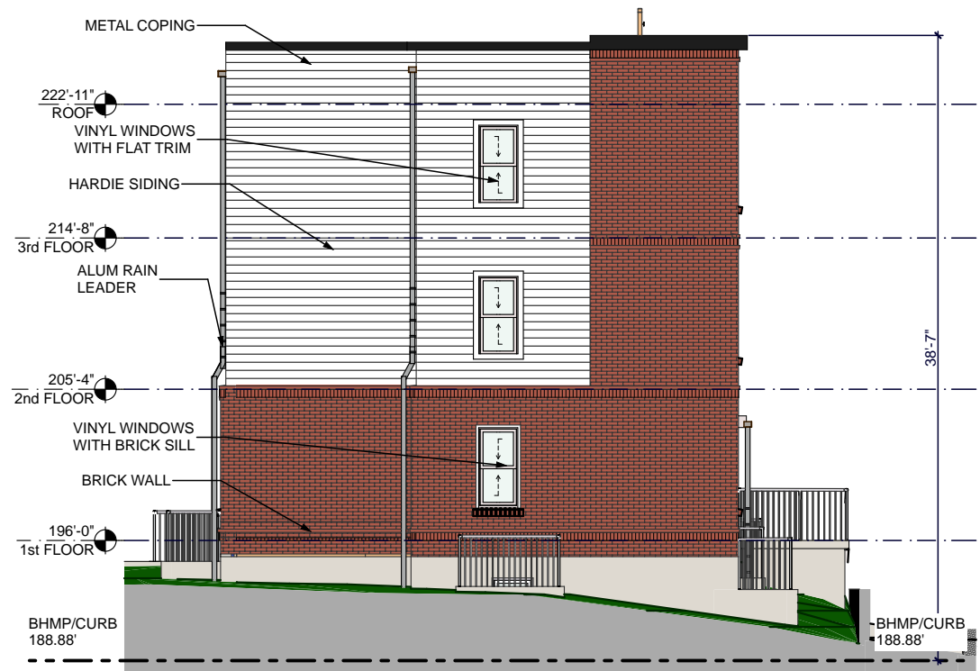
1 SOUTH ELEVATION SCALE: 3/32" = 1'-0"
